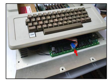
5. Unplug the keyboard connector from the motherboard. This is easily accomplished using a small flatbladed screwdriver but must be performed carefully to ensure that the connector does not get damaged in the process.
