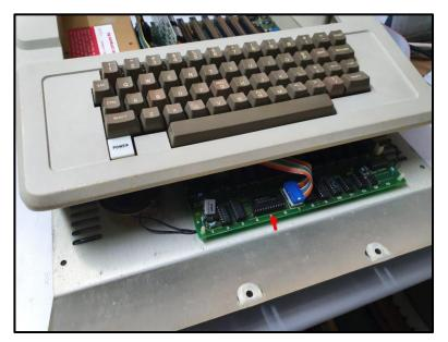
5. Working around the keyboard connector, remove the 2316B SPCL ROM at position A5 from its socket.
