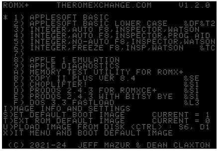
2. Press 1 to boot using the regular Applesoft Basic ROM. If you have the optional ROMX text ROM, try pressing the 2 key to boot using the lowercase modified Applesoft ROMs whilst simultaneously switching to font 2. All going well you should see the APPLE ][ Boot logo displayed in lower case as below :
