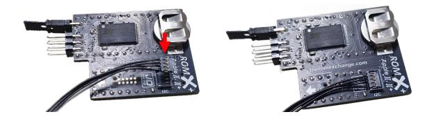
To disconnect the I2C cable, grip the wires and gently pull the cable directly upward :
