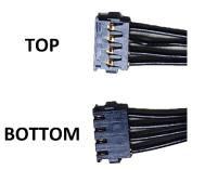
Then line the connector up directly above the socket, and apply light pressure to seat it. It should click into position :
